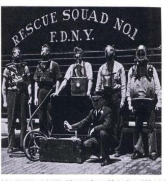
Left to right: 2 Hose Masks; M.S.A. Self-contained Orygen; All-Service; Draeger Self-Contained Breathing Apparatus; Center—Captain Millner operating blower which supplies the Hose Masks
